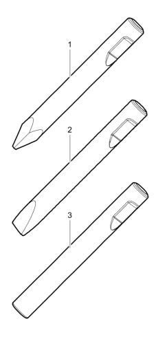
Ø=135 mm, L=640 mm, L $_{\rm T}$ =1125 mm, Wt=111.8 kg Ø=5.31 inch, L=25 inch, L $_{\rm T}$ =44.29, Wt=246.5 lb
