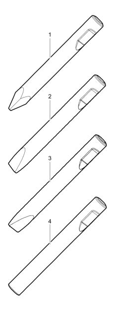
Ø=135 mm, L=635 mm, LT=1125 mm, Wt=111.0 kg Ø=5.31 inch, L=25 inch, LT=44.29 inch, Wt=244.7 lb
